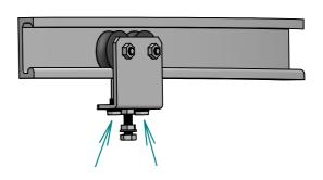
Hang the door to the runners using the door brackets
