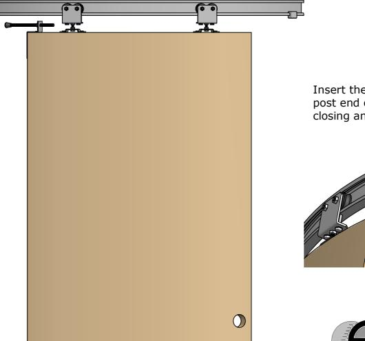
Insert the door stop at the door post end of the track, adjust for closing and lock into position
